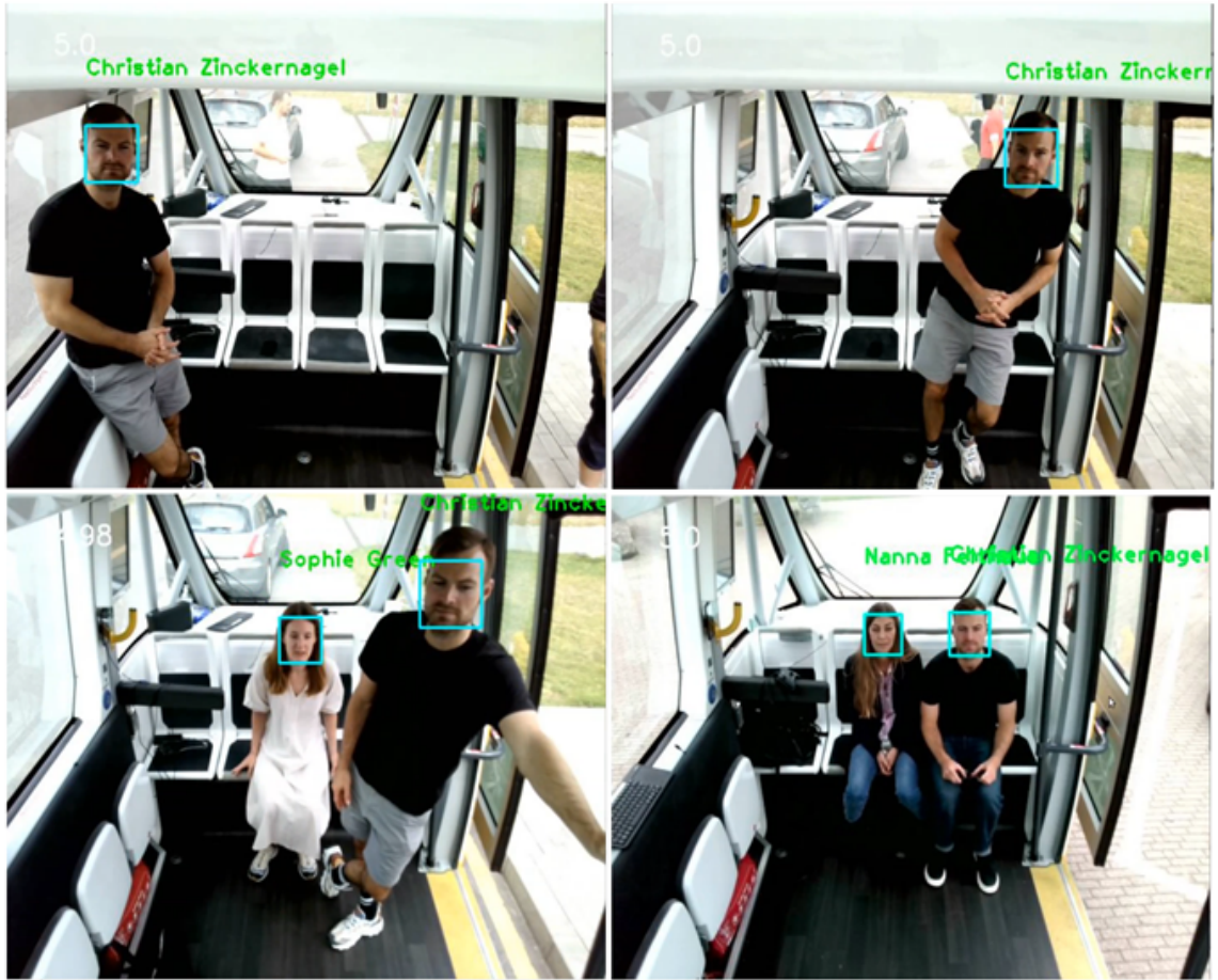
Figure 4.43: An experimental real-world demonstration running on the NVIDIA Jetson AGX Xavier. The proposed system is able to correctly identify the two passengers of the autonomous shuttle, among a database of 20 people.
