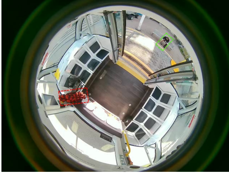
Figure 4.35: Illustration of a false positive: the green bounding box represents a correctly identified individual, whereas the red bounding box indicates a false positive detection by the algorithm, misidentifying a piece of cloth as a person. This example highlights the challenges in discriminating between actual human figures and objects with similar form factors in complex visual scenes.
