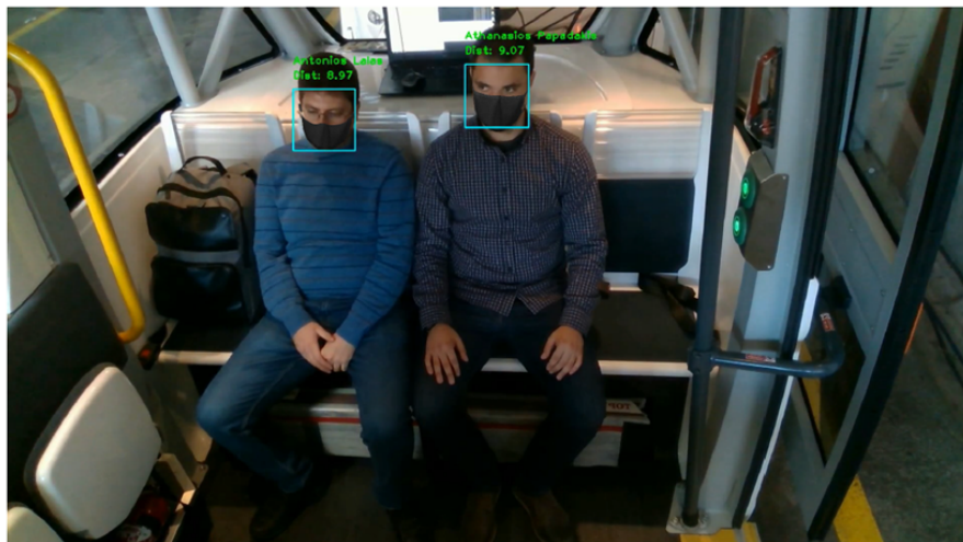
Figure 4.42: An experimental real-world demonstration running on the NVIDIA Jetson AGX Xavier. The proposed system is able to correctly identify the passengers of the autonomous shuttle even with their face masks on, among a database of 10 people.
