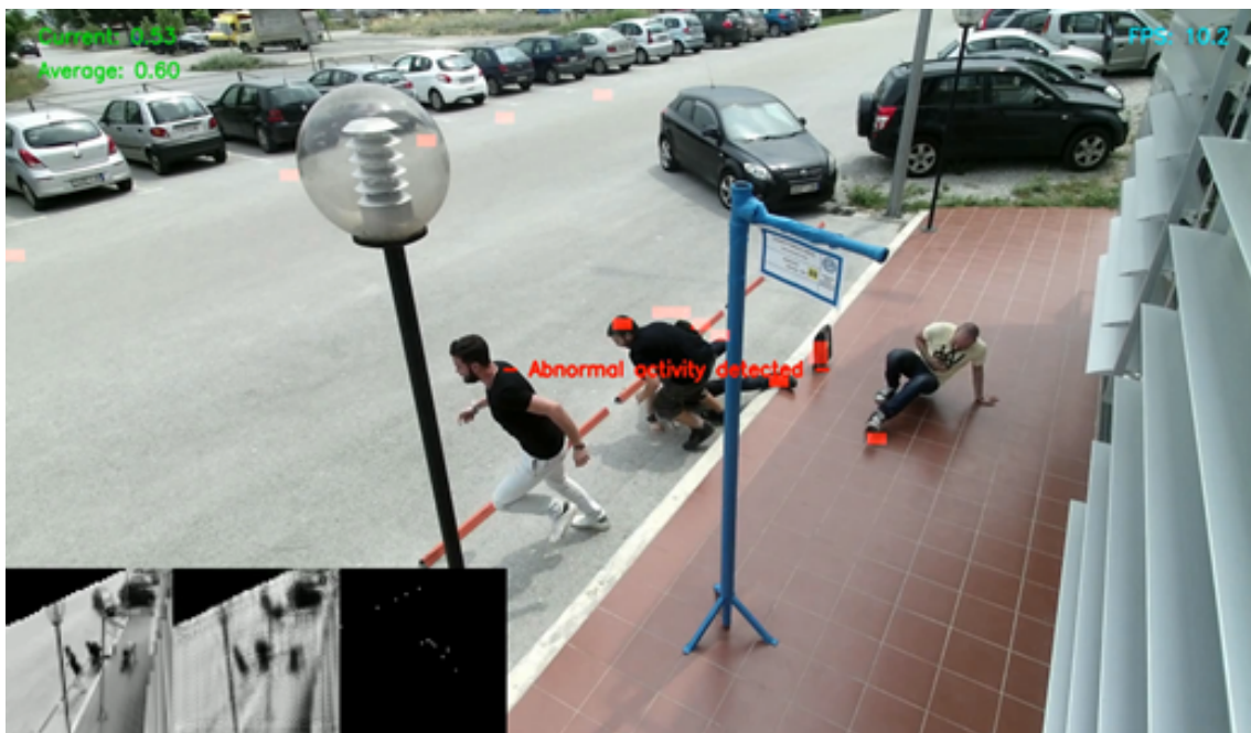
Figure 4.19: Evaluation on UC01 (fighting event) illustrating a group of four people injured on the ground and running. The images in bottom-left side illustrate the network's input, the reconstructed input and their absolute difference map.
